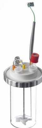
Sample sizes up to 100ml, mechanically stirred. Available for the 4 or 8 reactor block version (left).
