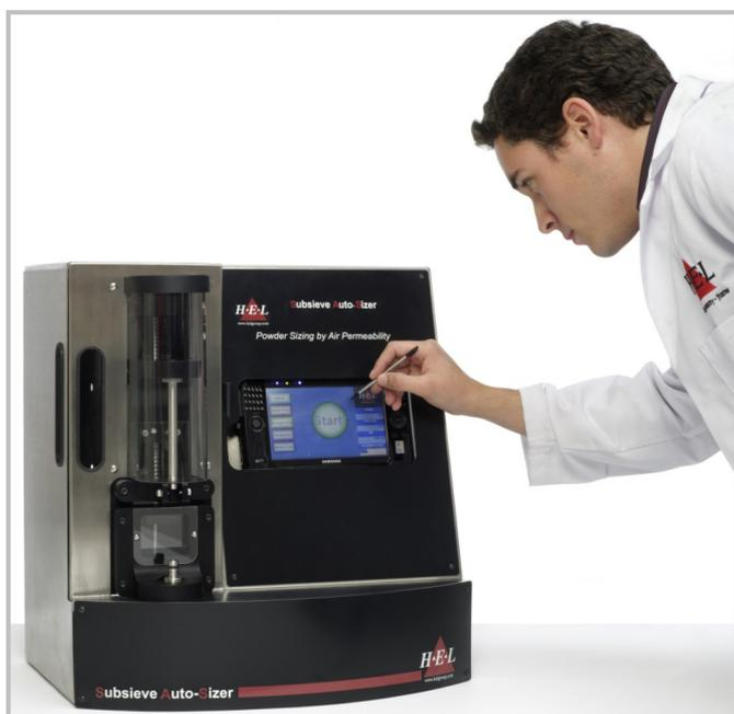
Developed as a direct and improved successor to the widely used Fisher Model 95 Sub-Sieve Sizer (FSSS), HEL have improved on the FSSS's performance and brought the technology to the 21st century by offering easy to use automated functions together with electronically recorded data.
