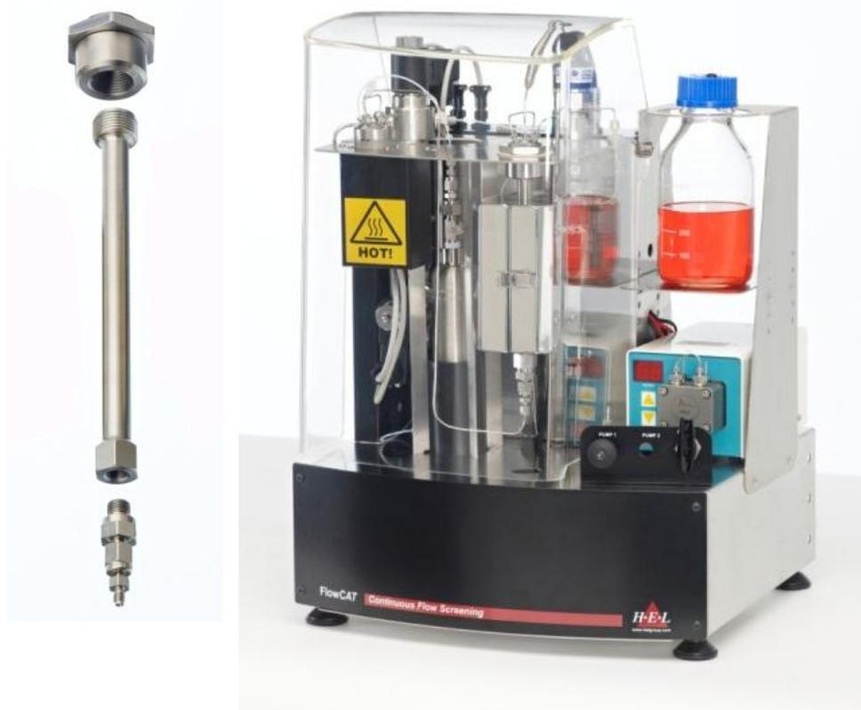
Tubular reactors are either 6mm (1/4”) or 12mm (1/2”) diameter though can be larger and the length is normally 15cm of which 10cm is the temperature controlled (hot) region. This gives a maximum hot zone reaction volume of approximately 3 and 12ml respectively. These specially machined reactors can be easily replaced by coiled tubing and used in the heated zone where the chemistry favours this alternative reactor type.
