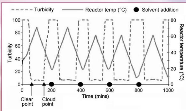
Figure 2 – Automated metastable zone width (MSZW) data reported by AstraZeneca
